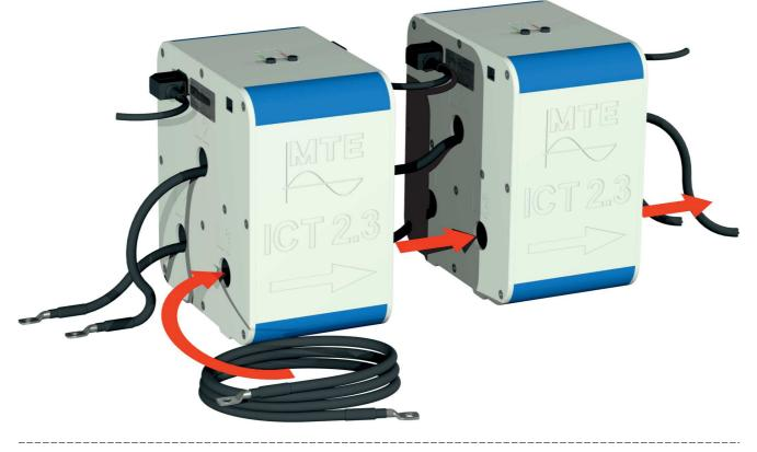
Passing the secondary current cables phase per phase through the corresponding holes. The length of the cables is adapted for use in direct connection or via ICT 2.3.
