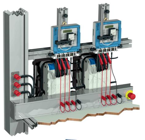
Connect auxiliary supply individual to each ICT 2.3 or connect to the first one and pass from ICT to ICT with interconnection cables. Pass the primary current cable phase per phase through the corresponding holes of the isolation current transformer ICT 2.3 and connect them at the current terminals of the test bench. The types of primary and secondary current cables needed depend on the type of the test bench and must be defined at time of order.
