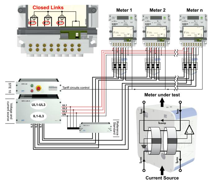
The ICT 2.3 performs the 1:1 current transformation with 1 winding by passing the primary and secondary current cable through the same hole. A big advantage of the connection through a hole is, that the same secondary current cables can be used for operation with ICT or for direct connection.
