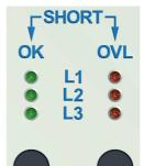
The SHORT activate the manual short circuit function. This function works on all phases at the same time and is useful, if not all measurement positions are used.
